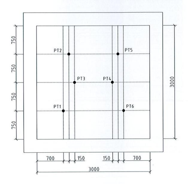
PT1-PT6: Thermocouples in the furnace
